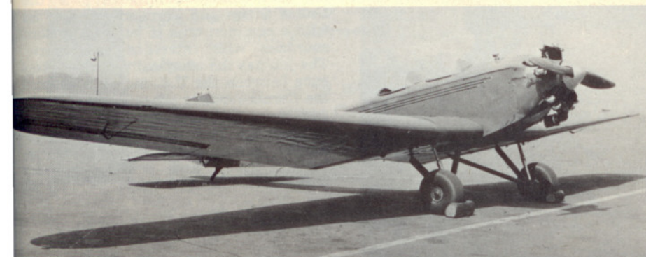
Aeromarine-Klemm AKL-26A had five horsepower more than AKL-26 and carried more fuel at a higher gross weight. Among the refinements added to this 1929 version were the new Goodyear Airwheels and lighting for night flying.
