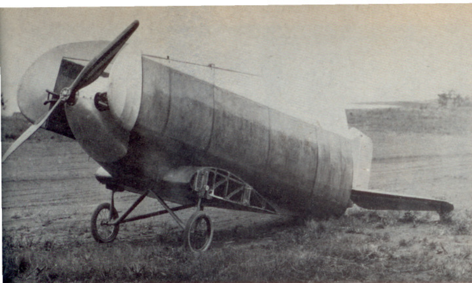
German Klemm L.25 with wings detached and stowed. Wing is plywood covered ahead of the rear spar for torsional stiffness. Fabric covered wingtip pivots to assist aileron function. Note large diameter of propeller on two-cylinder Daimler-Mercedes engine.
