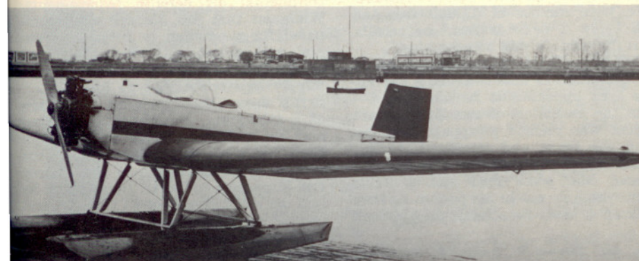
The generous wingspan of the Aeromarine-Klemm made seaplane operation possible on very low horsepower. This is Aeromarine-Klemm AKL-26, also known as AKL-60, with 60 h.p. LeBlond, one of several small American engines introduced during the 1928 aviation boom.
