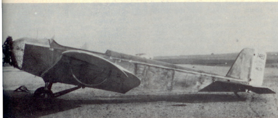
One of the earliest Aeromarine-Klemms, the AKL-26, with single cockpit for two occupants, wing tip skids, the pivoting wingtips, and wire wheels without brakes. Note wrinkling of the birch plywood used to cover the fuselage and vertical fin.
